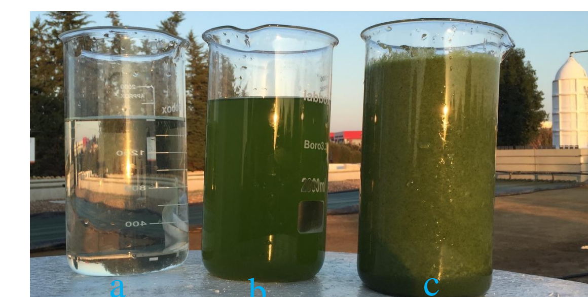
Figure 7 : Clarified water (a), algae effluent (b) and algae sludge (c)
